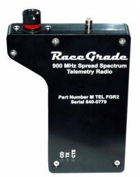
Frequency: 902-928 MHz spread spectrum Output Power: up to 1 Watt Sensitivity: -110dBm Baud Rate: up to 115.2 Kbps RF Connector: SMA female Supply Voltage: 6 to 30 VDC -20° to 75° C Temp. Range: Weight: 202 grams Compatible with any RS232 serial stream of data from different logger manufacturers.
