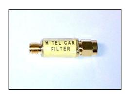
Note: Please prevent the housing or connectors from touching chassis ground or anything which conducts electricity like carbon fiber. The filter is wrapped in shrink help isolate the unit from noise.
